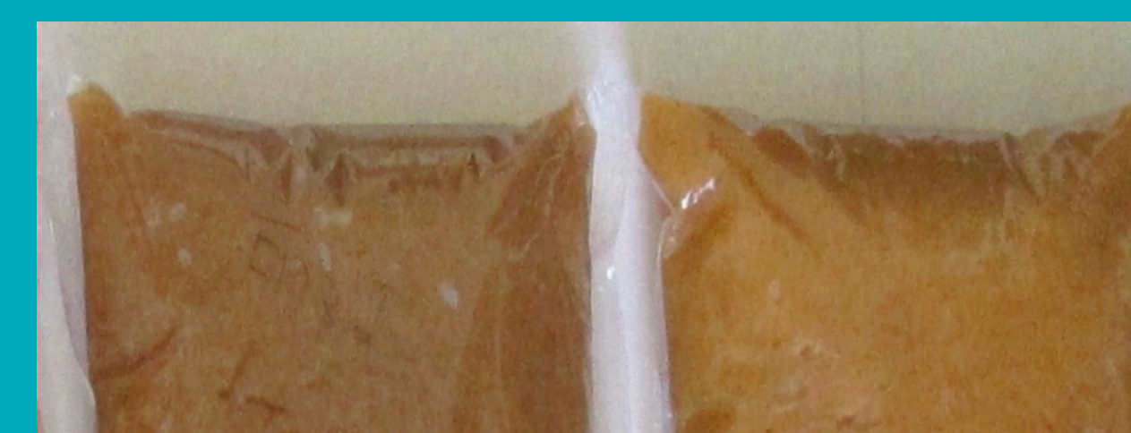
A. Untreated softwood pulp B. Softwood pulp treated with un-concentrated culture supernatant containing recombinant HLE peptide fused to a peptide of \beta -galactosidase. Note color change to lighter, more orange brown.
